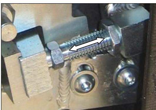
7.) Position the adjustment screw (3) in that way, which the door closes in the middle position.
