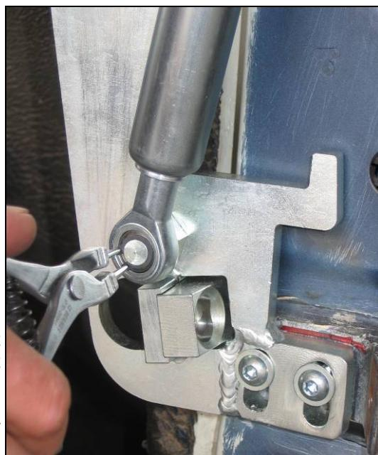
10.) Carefully pivot the door up and hang in the gas spring at the fitting point of the chassis plate. Secure it also with the supplied security ring.
