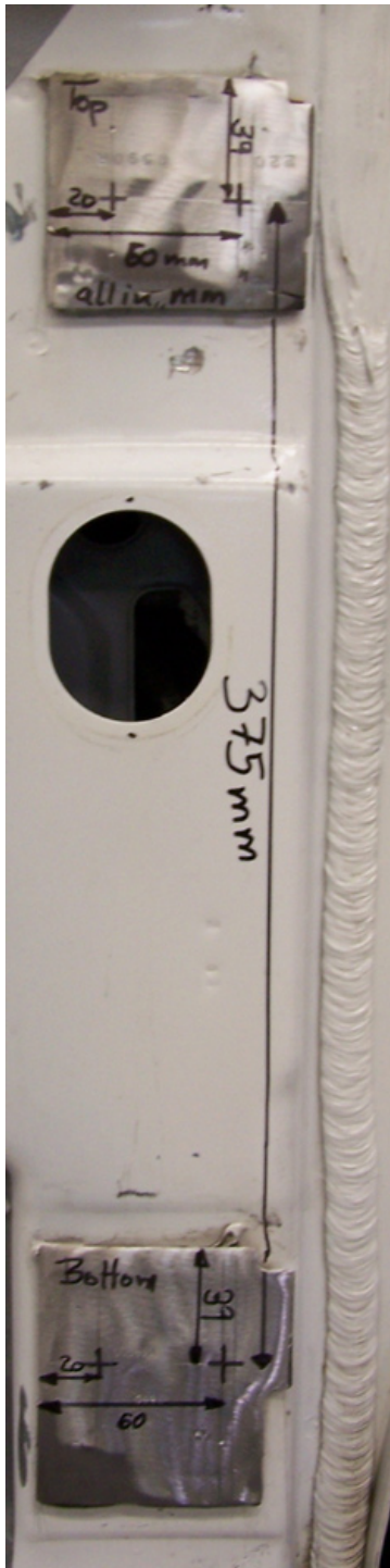
Top chassis hinge drill pattern
