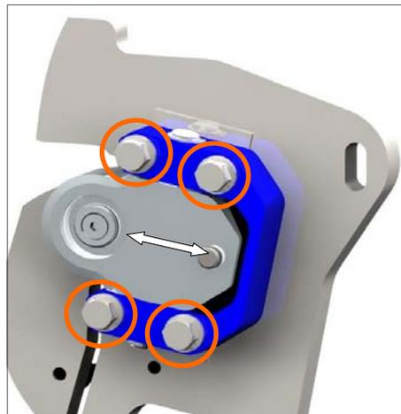
10.) Attach the swing arm to the ground plate with the 4 included bolts and adjust the door via moving the swing arm to chassis plate adjustable (2) connection mount with horizontal door gap adjuster (2) in the right or left direction until gap measurement is like original.
