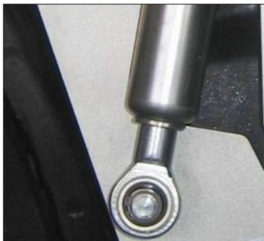
21.) Carefully pivot the door up, place in the gas spring (T) on the according mounting point on the chassis plate. Secure it with the supplied security ring.
