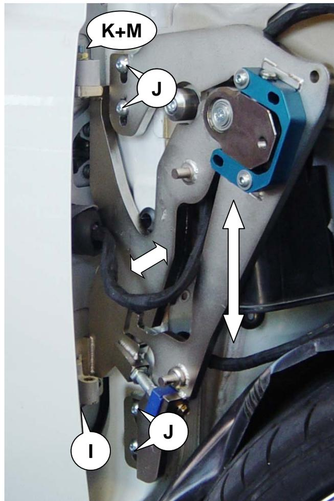
12.) Adjust the **height** of the door by moving the ground plate (**S**) vertically. You might have to loosen bolts (**J**) on the ground plate to do this.
