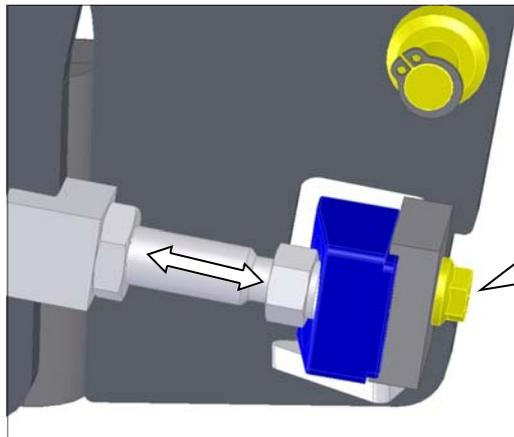
11.) Position the lower adjustment screw, MAGIC STICK (1) in that way, which the door closes in the center position.
