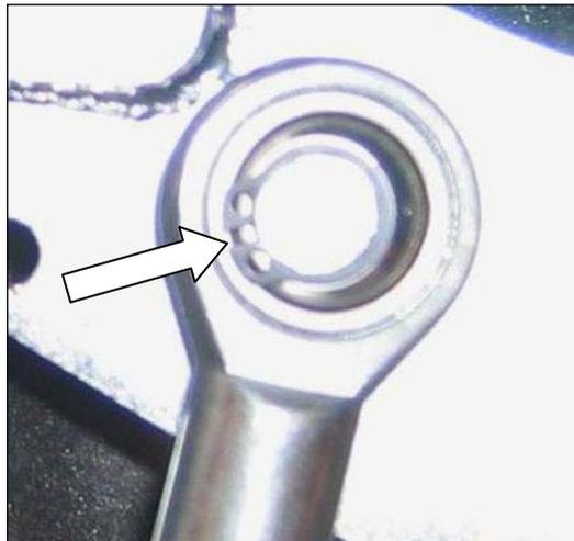
20.) Hang in the gas spring (T) on the fitting point of the swing arm. Secure it with the supplied security ring, by means of needle-nosed pliers.
