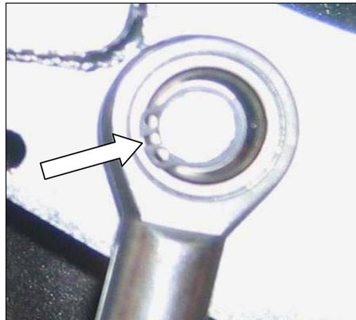
23.) Hang in the gas spring (U) on the fitting point of the swing arm. Secure it with the supplied security ring, by means of needle-nosed pliers.
