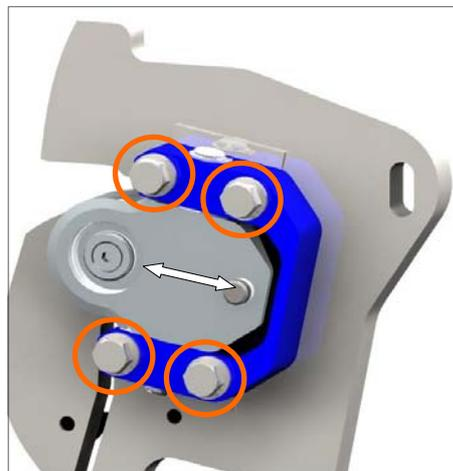
13.) Attach the swing arm to the ground plate with the 4 included bolts and adjust the door via moving the swing arm to chassis plate adjustable (2) connection mount with horizontal door gap adjuster (2) in the right or left direction until gap measurement is like original.
