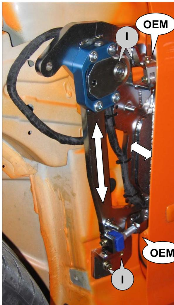
15.) Adjust the **height** of the door by moving the ground plate (**T**) vertically. You might have to loosen bolts (**I**) on the ground plate to do this.
