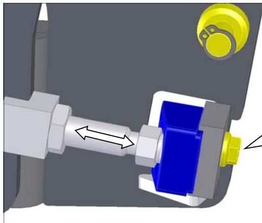
14.) Position the lower adjustment screw, MAGIC STICK (1) in that way, which the door closes in the center position.
