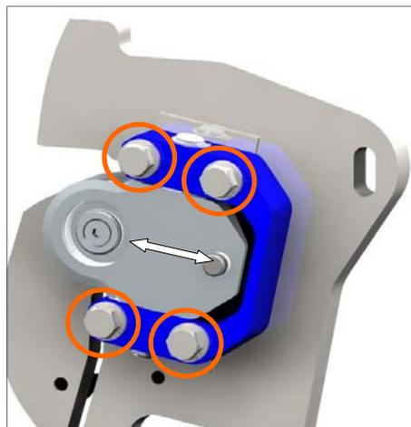
6.) Attach the swing arm to the ground plate with the 4 included bolts and adjust the door via moving the swing arm to chassis plate adjustable (2) connection mount with horizontal door gap adjuster (2) in the right or left direction until gap measurement is like original.
