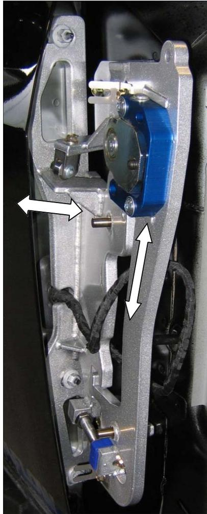
8.) Adjust the **height** of the door by moving the ground plate **(R)** vertically. You might have to loosen bolts **(G)** on the ground plate to do this.
