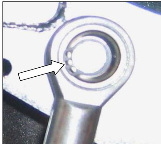
10.) Hang in the gas spring (**J**) on the fitting point of the swing arm. Secure it with the supplied security ring, by means of needle-nosed pliers.
