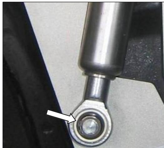
11.) Carefully pivot the door up, place in the gas spring (**J**) on the according mounting point on the chassis plate. Secure it with the supplied security ring.
