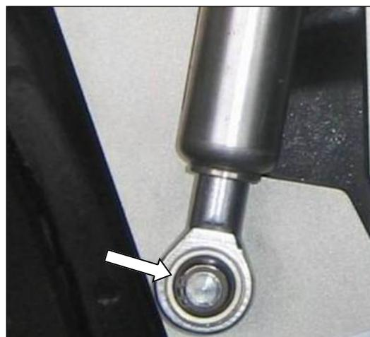
18.) Carefully pivot the door up, place in the gas spring (O) on the according mounting point on the chassis plate. Secure it with the supplied security ring.
