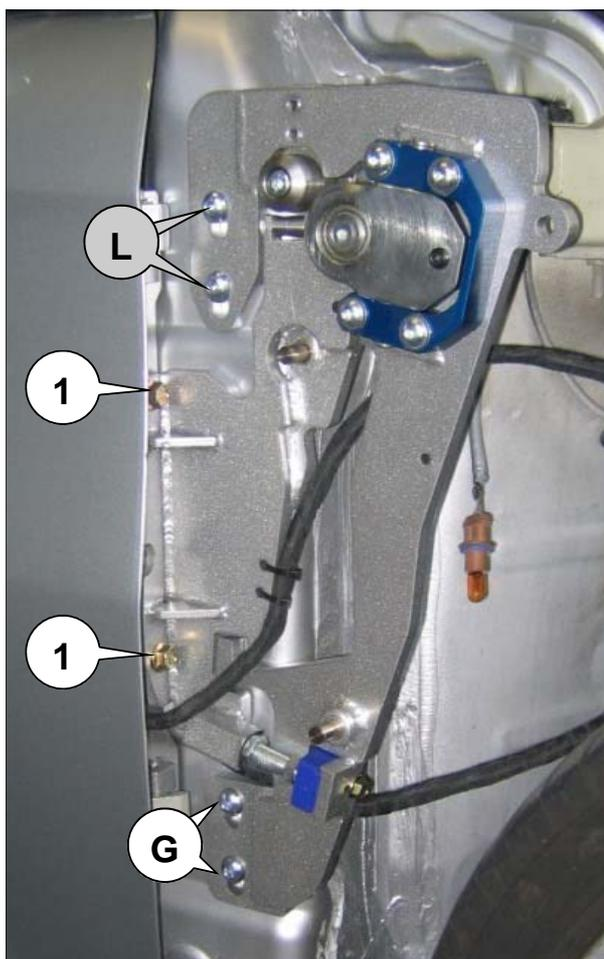
13.) Adjust the **height** of the door by moving the ground plate **(R)** vertically. You might have to loosen bolts **(L)** on the ground plate to do this.
