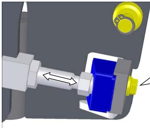
12.) Position the lower adjustment screw, MAGIC STICK (1) in that way, which the door closes in the center position.
