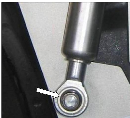
16.) Carefully pivot the door up, place in the gas spring (**J**) on the according mounting point on the chassis plate. Secure it with the supplied security ring.
