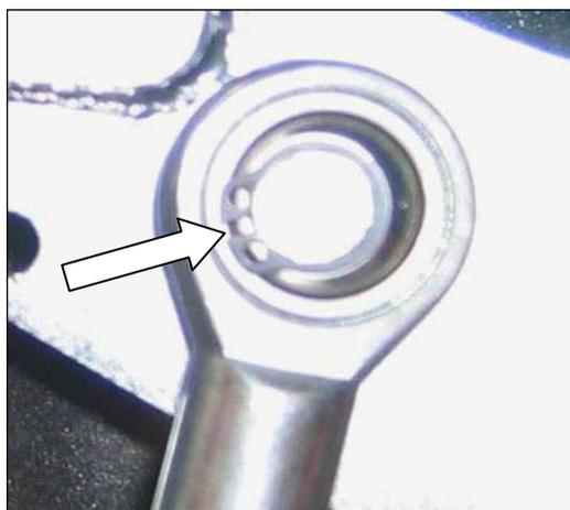
15.) Hang in the gas spring (**J**) on the fitting point of the swing arm. Secure it with the supplied security ring, by means of needle-nosed pliers.
