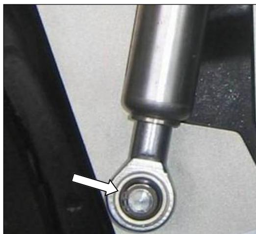
17.) Carefully pivot the door up, place in the gas spring (V) on the according mounting point on the chassis plate. Secure it with the supplied security ring.
