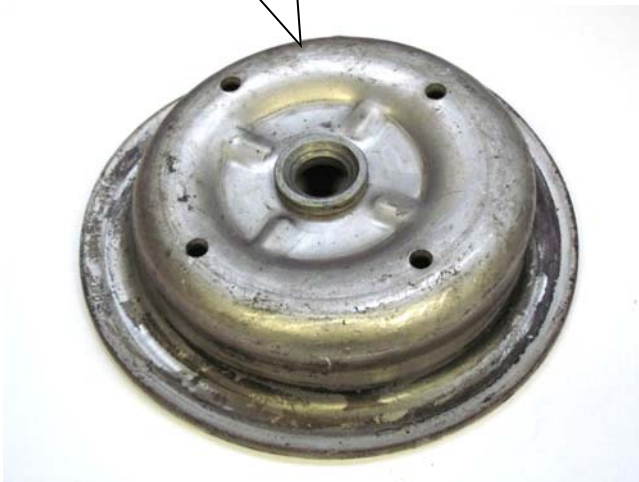
Aluminiumfederteller Aluminum spring perch.
