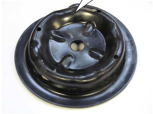
Stahlfederteller Steel spring perch.
